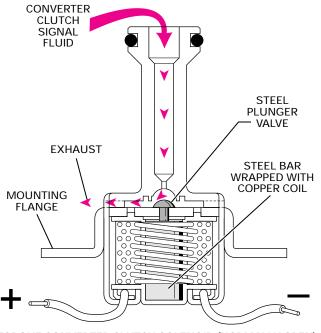
TORQUE CONVERTER CLUTCH SOLENOID (NORMALLY OPEN)
