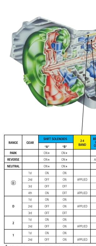
SOLENOID "A" & "B" OPERATION AND THE SHIFT VALVE POSITIONING IN P.R.N. RANGES ARE A FUNCTION OF THE INPUT TO THE SOLENOIDS FROM THE VSS. UNDER NORMAL OPERATING CONDITIONS THE SOLENOIDS ARE ON IN P,R,N.
