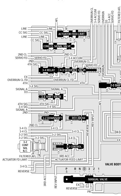
COMPONENTS LOCATED IN THE VALVE BODY
