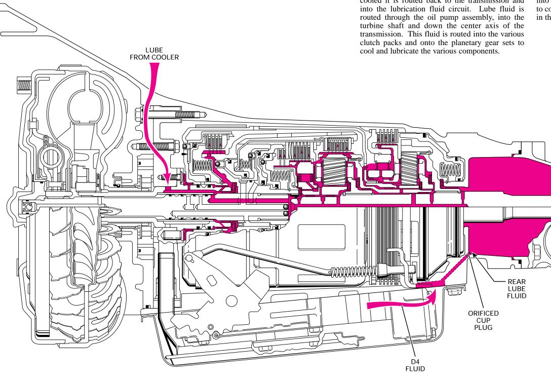
The rear of the transmission is lubricated by D4 fluid feeding the rear lube fluid circuit through an orifice cup plug (#24). Rear lube fluid is routed into the transmission case extension housing (31) to cool and lubricate the bushings and components in the housing.
