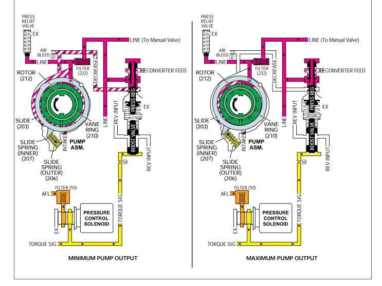
COMPONENTS LOCATED IN THE VALVE BODY
