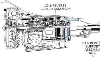
The lo and reverse clutch assembly is located in the rear of the transmission case and is applied in Park, Reverse and Manual First - First Gear. The steel clutch plates (682A,B,D) are splined to the transmission case while the fiber clutch plates (682C) are splined to the reaction planetary carrier (681). When applied, the lo and reverse clutch plates hold the reaction planetary carrier stationary to the transmission case.
